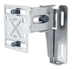
Fastening panel for mounting device installation trunking on skirting board constructions and as a support for the convection grid. The fastening panel can be used for all Rapid 80 device installation trunking systems of type GK and GA. When mounting plastic GK device installation trunking, the matching wall panel adapter is also required. The connection profile is required for mounting double trunking of type GS-D70170 and GS-D90170, as well as for GS trunking with a nominal width of 210 mm.
